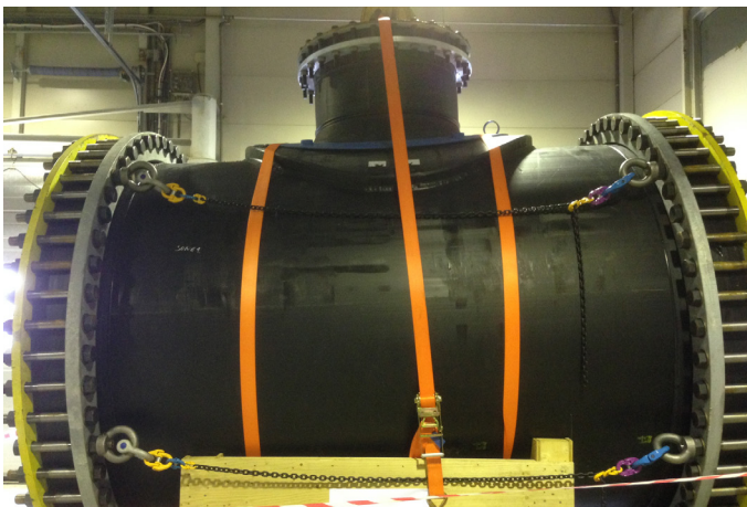
Full scale pressure test of OD1000 saddle on OD2500 pipe to 2 bar
