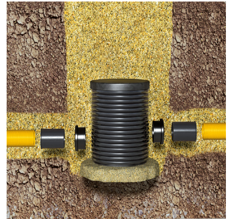
Sample installation of an underground drainage chamber.
