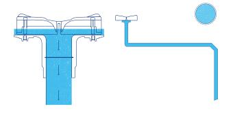
Siphonic outlets utilize air baffles to prevent air from entering the pipeline and inhibit the formation of the vortex.
