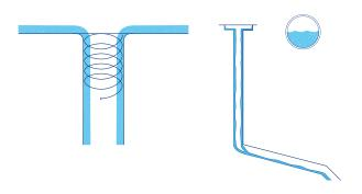
Conventional rainwater drainage systems utilize gravity to draw water into the downpipes. However, this also allows air to enter, causing the water to vortex along the pipes walls and reduce drainage flow rates.
