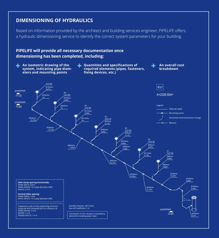
Deviations from the original documentation (e.g., changes in pipe lengths or diameters) must have written consent from PIPELIFE before being implemented.
